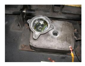
With the parts cleaned, I put the conversion gear on the new moter, this is a very tight fit and is machined to fit with no play. Care is needed when it is tapped back on the new motor gear so you don't misalign the pin and the gear.
