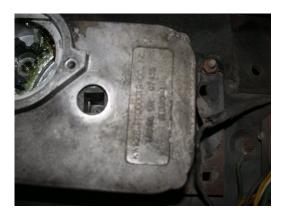
Next I put the linkage back into place and put the linkage bushing back into the cover plate.
