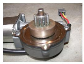
With the step linkage taken out of the gear box, I marked one side of the square in the linkage hole in the center, cleaned out the old grease, checked for any damaged teeth and put new grease in the box next I re-indexed the main gear turning it 180 degrees using the marked square in the center of the gear as a guide.
