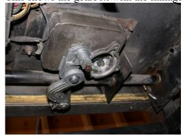
The linkage pulled from the gear box.
