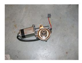
Next place the motor locating pin in the top of the conversion gear. This pin goes into the hole on the top of the gear box.
