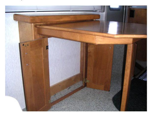
3. Remove the top. Looking straight up locate the 4 screws holding the top to the cabinet and remove:
