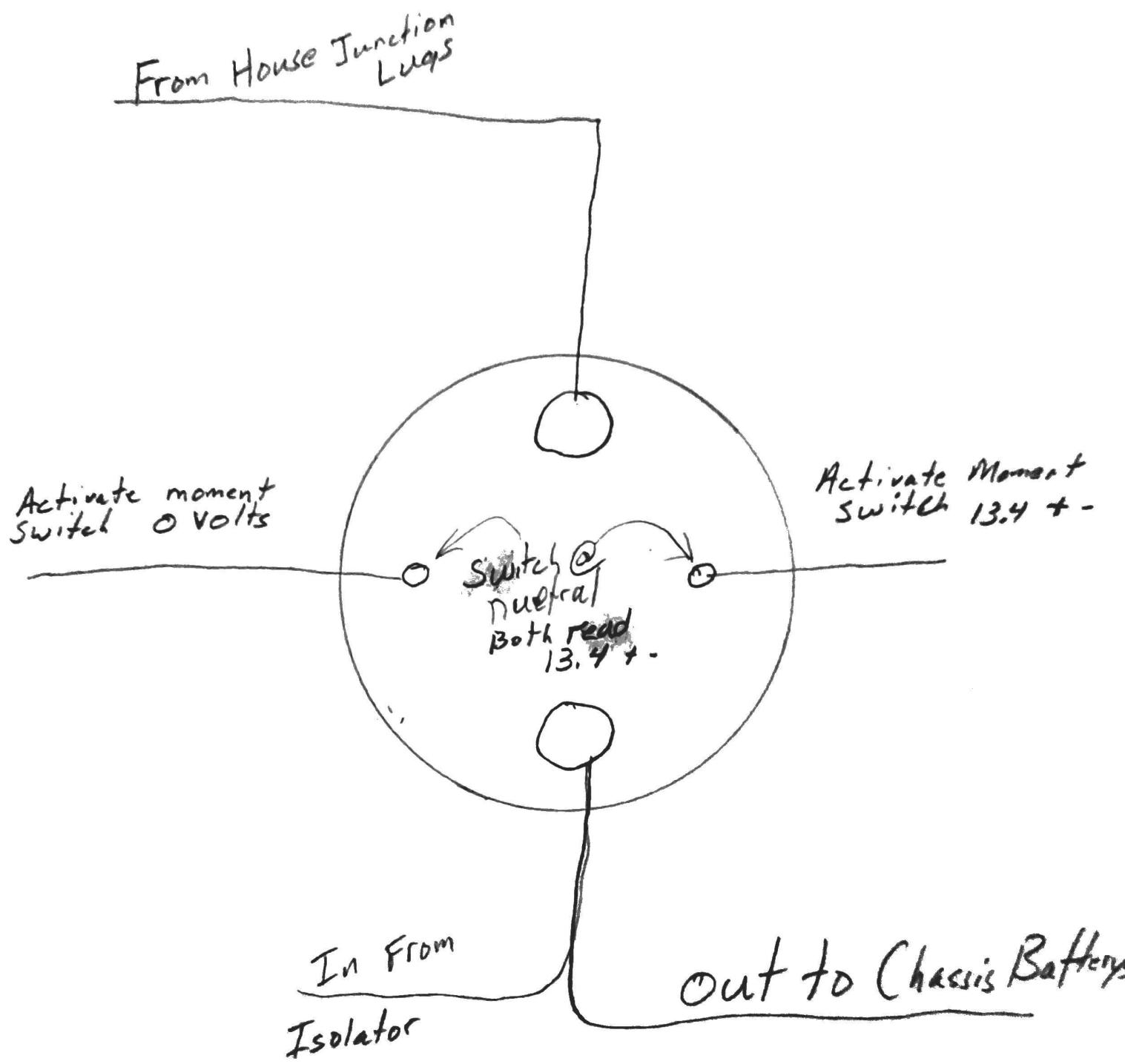
When Switch is pushed chassis and house lugs read equal voltage so solenoid is working
