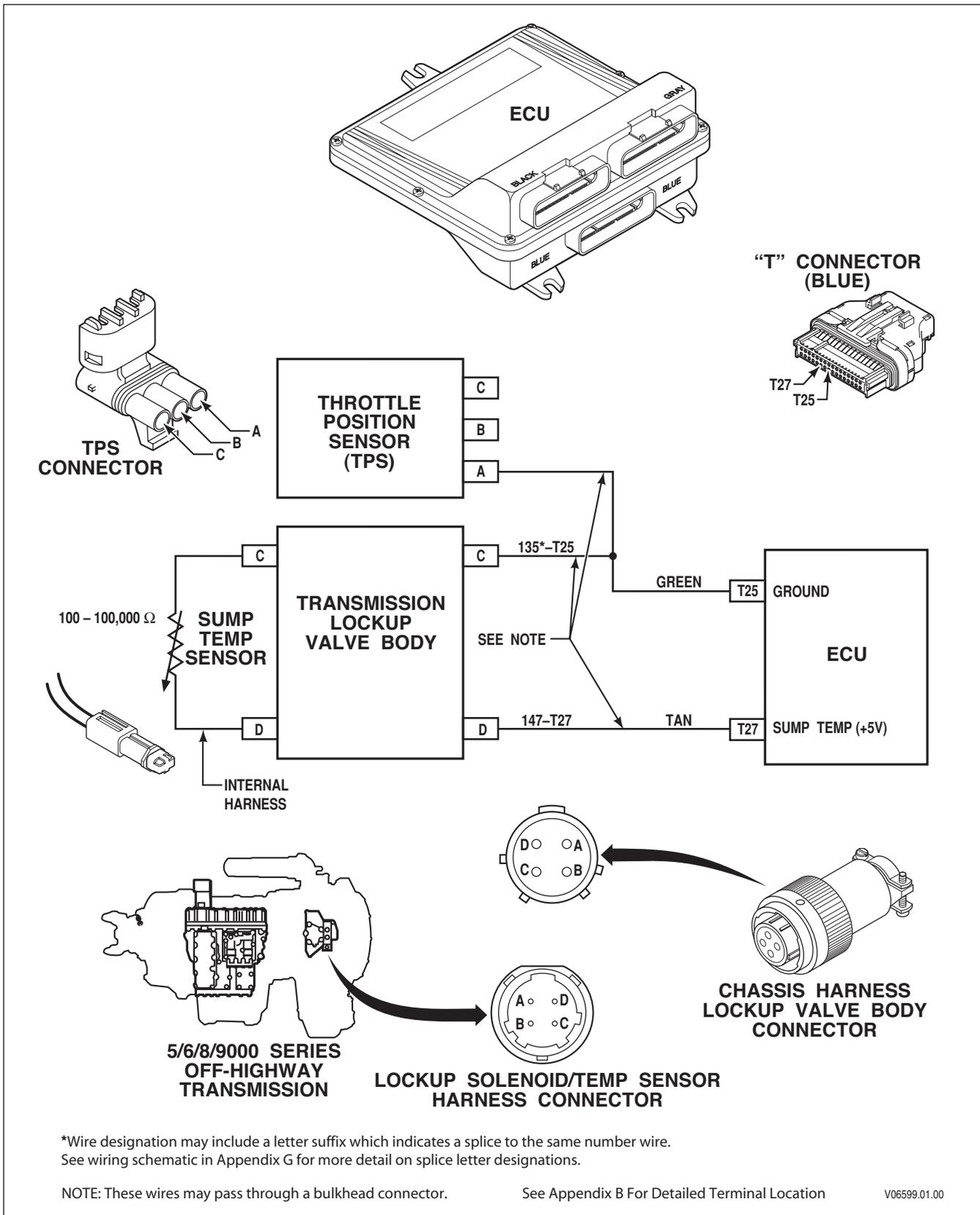
**Figure 5–8. Code 33 Schematic Drawing**
