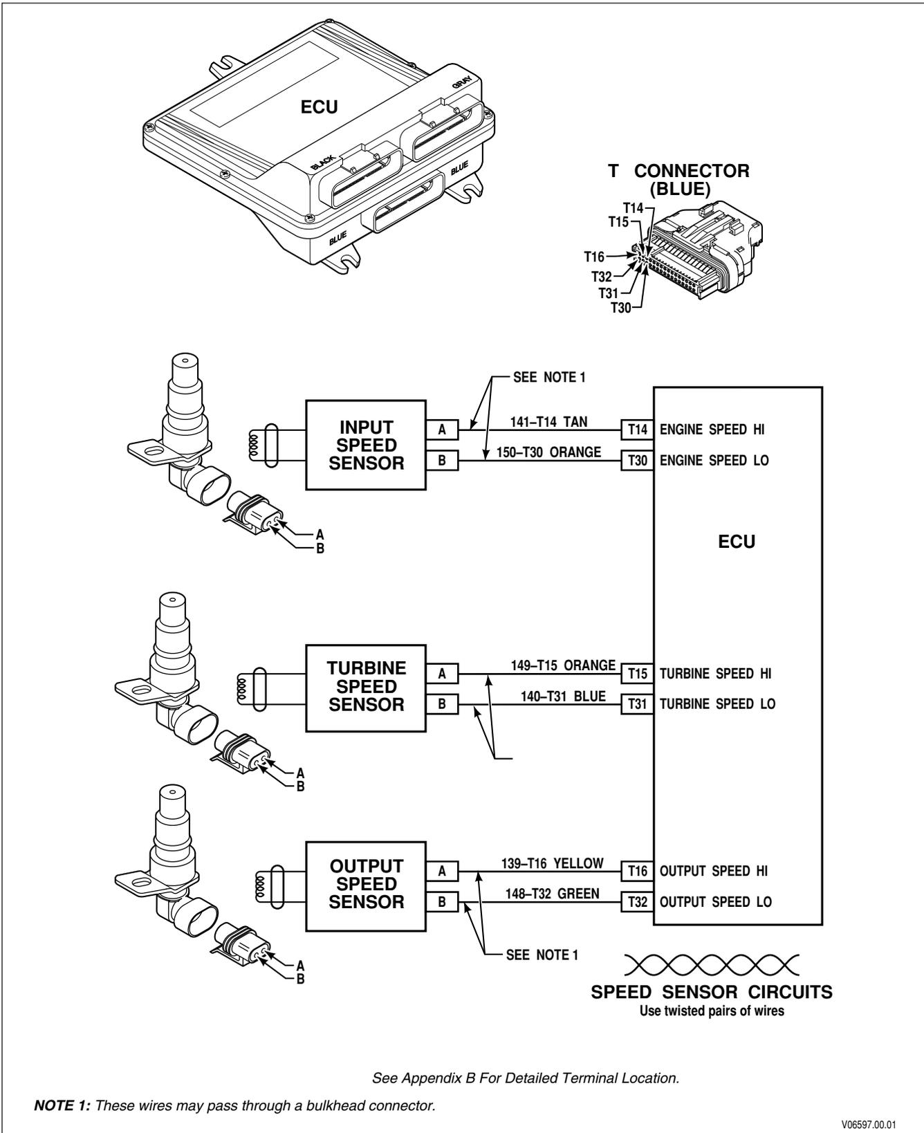
Figure 5-7. Code 25 Schematic Drawing
